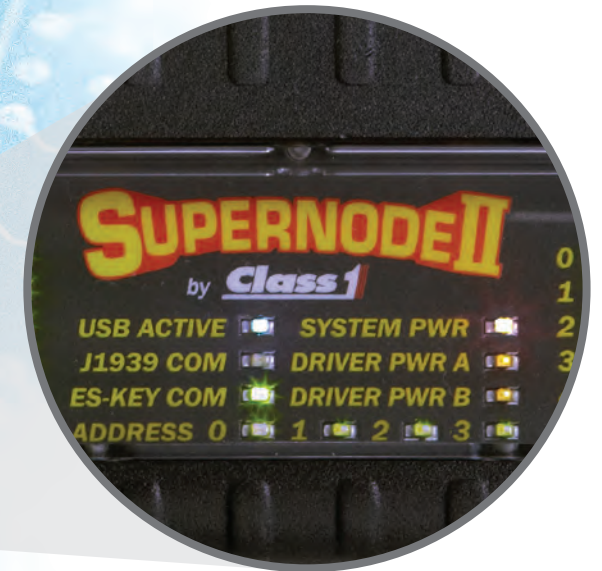
Input and Output LED status indicators
