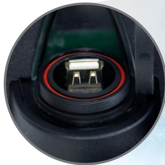
USB port for digital transfer and diagnostics
