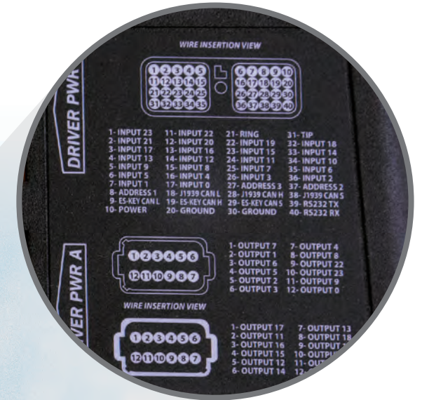
Integral power connectors for Duetsch and other connectors
